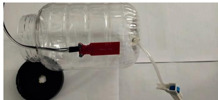
Figure 5: The container *cont1* with the pipe and the water-level sensor
