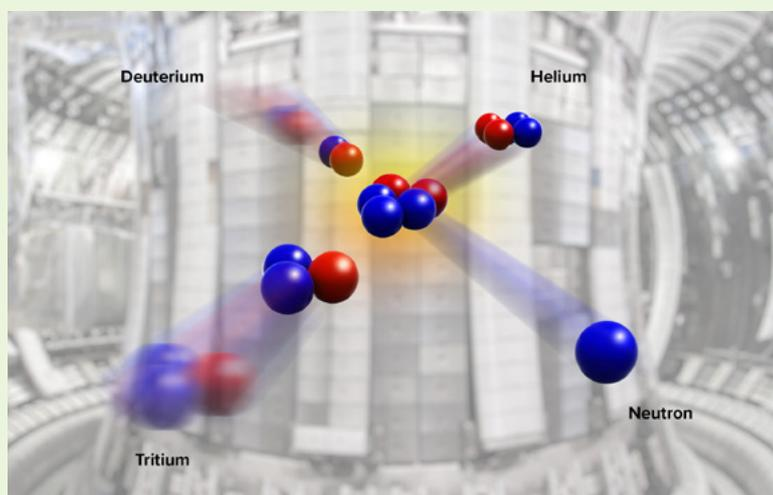
The fusion reaction  $D + T \rightarrow He + n + \text{Energy}$
