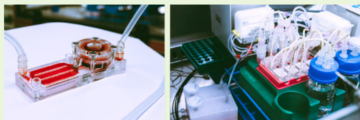
German Federal Institute for Risk Assessment. Left: single unit. Right: four units running in parallel connected to peripheral devices (pumps, sensors, reservoirs etc.)
