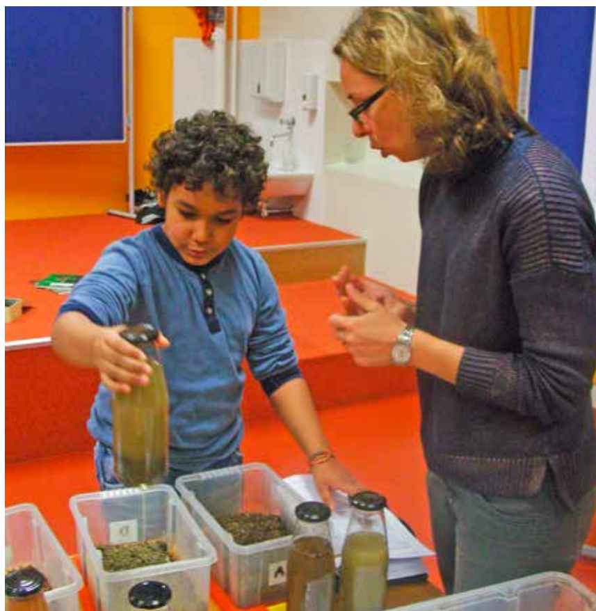
Shake it up: mixing the soil and water before letting it stand for 4 hours
