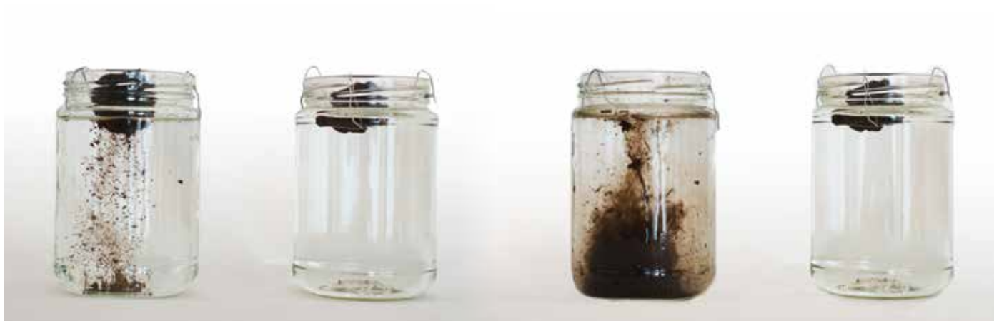
Figure 2: Soil samples immersed in water, after 1 minute. Soil from a disturbed site (left) and from the surface of an undisturbed site (right)
