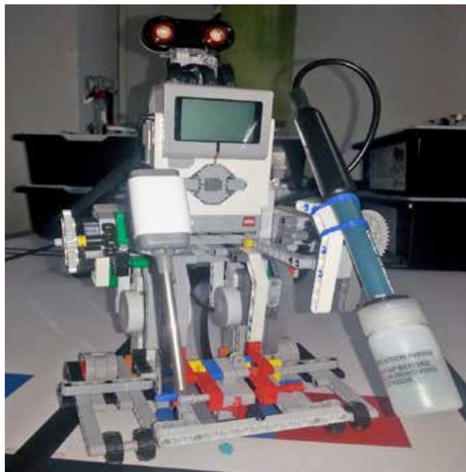
*A finished Chembot, complete with sensors*
