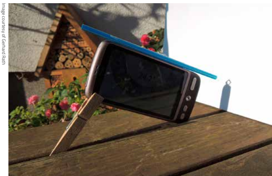
Figure 7. Measuring the Sun's elevation. When the shadow of the straw is at its smallest, the smartphone is correctly aligned.
