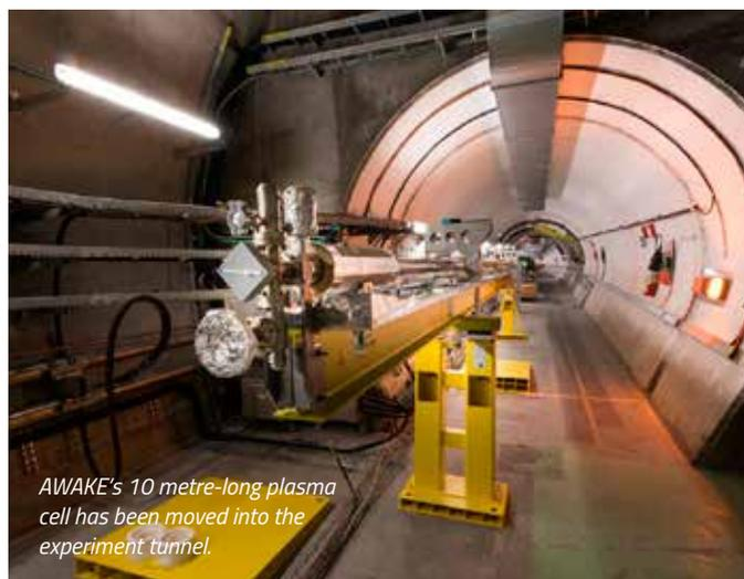
AWAKE's 10 metre-long plasma cell has been moved into the experiment tunnel.
