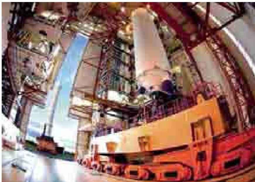
Solid rocket booster arrives for integration with the main cryogenic stage for Jules Verne's Ariane 5 ES launch vehicle
