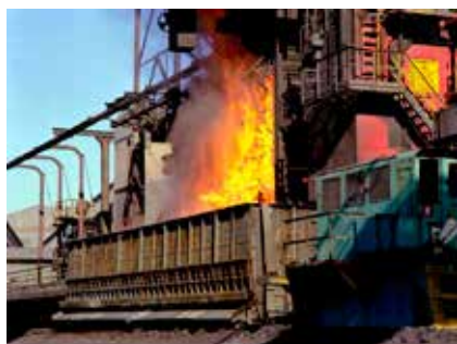
Coal is converted to coke in coke ovens. Thiocyanate ions are a by-product.
